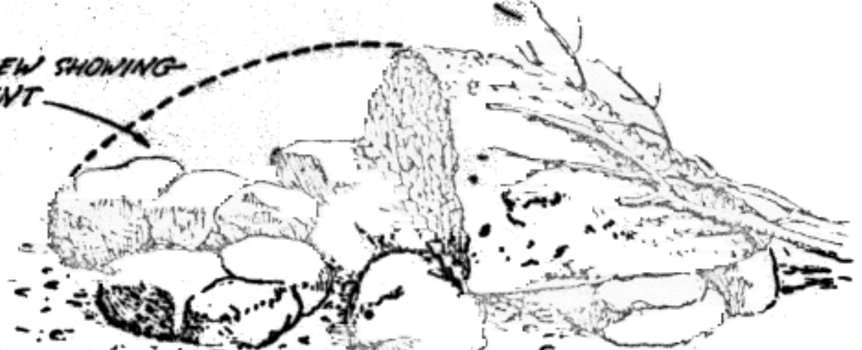
BUILD THIS RETREAT FOR RABBITS & FURBEARERS BY LAYING ROCKS AS SHOWN, COVER WITH FLAT ROCKS OR DISCARDED SHEET IRON TO FORM TUNNELS 6" HIGH. COVER WITH EARTH, STONES & BRUSH.
